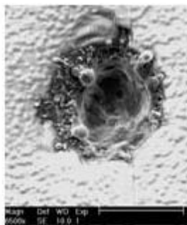
Figure 13. Example of thermal effects such as melting and splashing observed using ultrafast processing.
